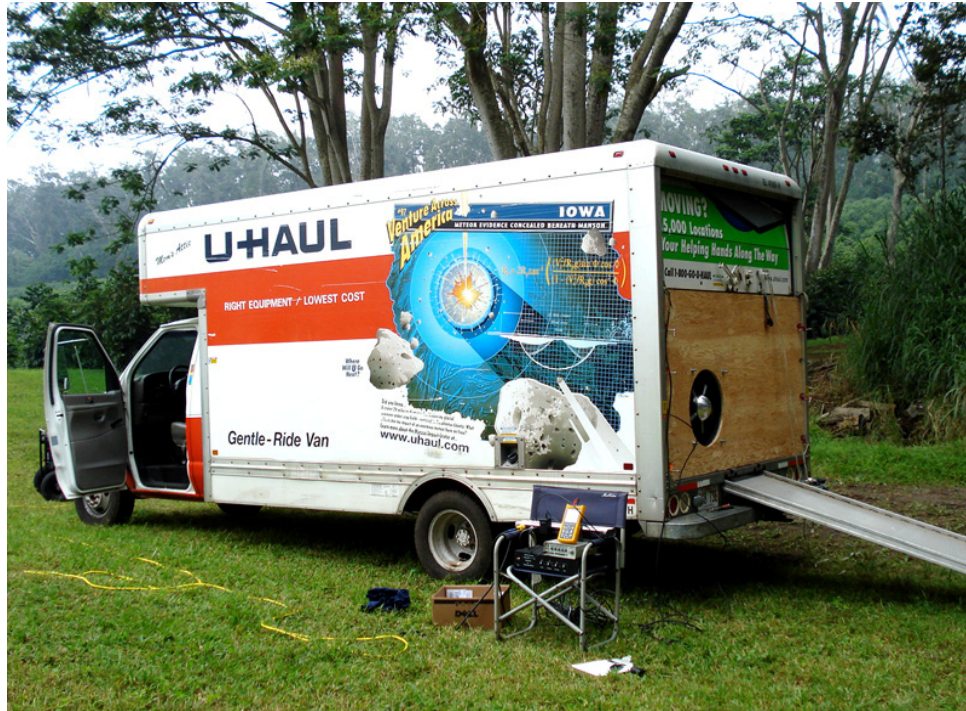
Figure 2. The Kona Infrasound Noise Generator in it's portable configuration, located approximately 3.8 km from the central element of I59US.
